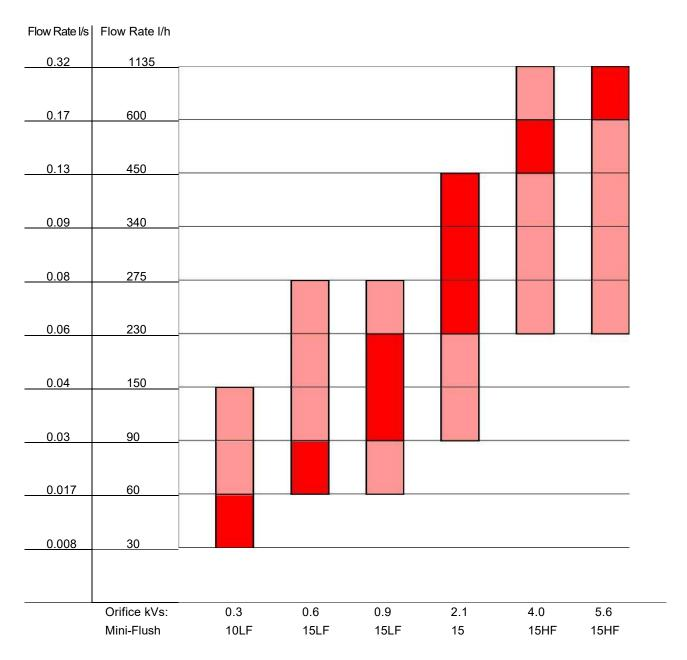
This chart is for guidance only. Any selections must be checked with a Tacotherm representative before a final selection can be made.
