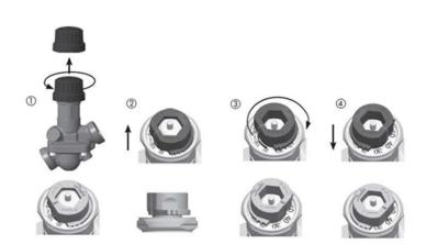
The presetting scale indicates values from 100 % flow to 0 %. Clockwise turning would decrease the flow value, while counter-clockwise would increase it.
